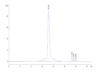
The purity of Biotinylated Human FcRH5 is greater than 90% as determined by SEC-HPLC.
